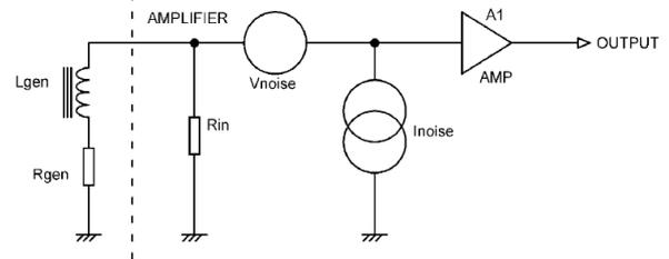
Fig. 2. The inductive source model
